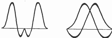
Fig. 12. Connecting the c.r.o. across a transformer or to an audio stage instead of the second detector produces a phase shift, pulling part of the pattern below the back-trace line and so distorting the pattern that it cannot be used.
